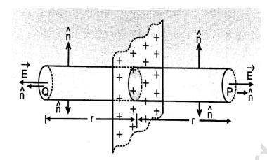
Draw a Gaussian cylinder of area of cross-section A through point P. The electric flux crossing through the Gaussian surface is given by,
