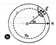
Hence, the field due to a uniformly charged spherical shell is zero at all points inside the shell. The variation of electric field intensity E with distance from the centre of a uniformly charge spherical shell is shown:
